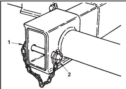
7. Install the retaining pin (1) through the grid and arm weldment and secure with the click pin (2).
