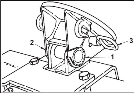
4. Install the 5th wheel plate onto the adapter with the attaching pin (1). Secure the attaching pin with the linchpin (2).
