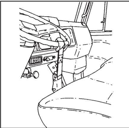
13. Always secure the steering wheel of the casualty vehicle with a steering wheel strap for any front or rear end tow.
