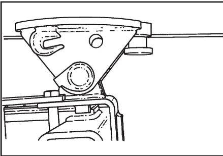
6. Extend the underlift boom and 5th wheel attachment up to the king pin of the casualty vehicle.
