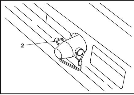
5. Install the pins into the outer sections of the outriggers.
