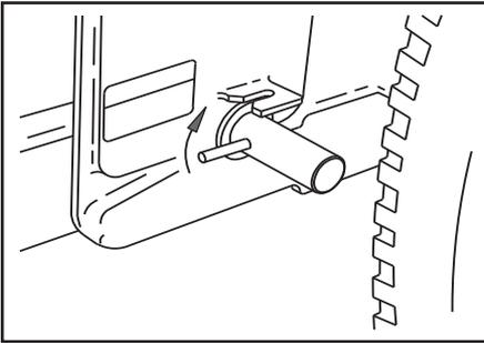
7. Install the pins into the outer sections of the outriggers.
