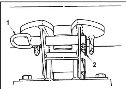
7. Engage the 5th wheel plate with the king pin. Install the king pin locking pin (1) and linchpin (2).
