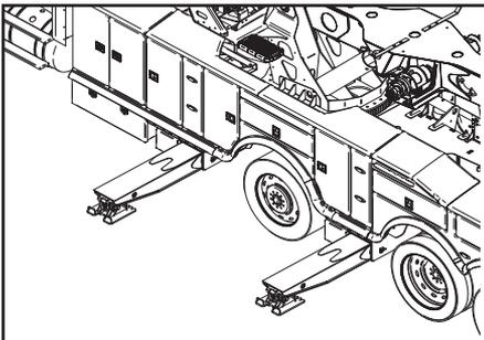
2. Using the controls, extend the outriggers to the full extended position.
