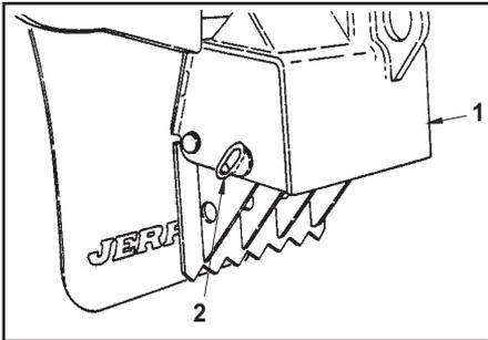
3. Line up holes and insert spade pin (2) and retaining pin (1).
