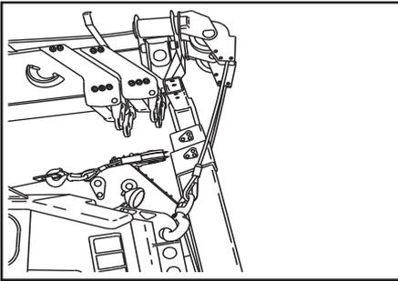
3. Unhook the wire ropes from their stored position. Moving the wrecker boom with the wire ropes hooked can result in damage to both the wire ropes and the boom.
