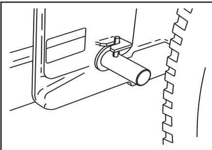
8. Rotate the pin to lock the pin keeper
