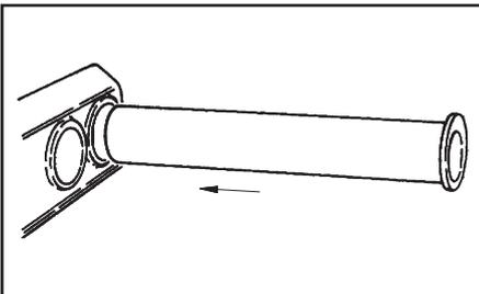
3. Insert the round tube into the desired position in the grid.
