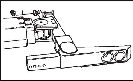
1. Remove the tire lift grid from the toolbox and slide the tire lift grid onto the crossbar. There are two width positions. The wider width would be used for wide front end lifts for example, and the narrow width would be used for narrower rear end lifts.
