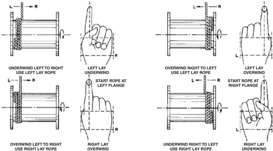
A simple method of determining how a wire rope should be started on a drum is shown above. The observer stands behind the drum, with the rope coming towards him. Using the right hand for right-lay wire rope, and the left hand for left lay wire rope, the clenched fist denotes the drum, the extended index finger the oncoming rope.
