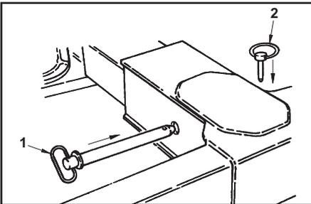
2. Install the retaining pin (1) from the back side of the crossbar through the grid and crossbar and secure with the pin (2).
