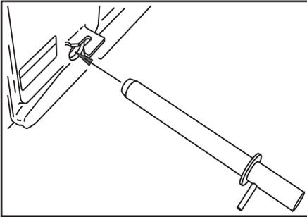
6. Lower the outriggers slightly to gain access to the pinning locations at the upper, inboard ends of the outriggers.
