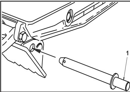
2. Line up holes and insert spade pin (1) and secure with the retaining pin (2).
