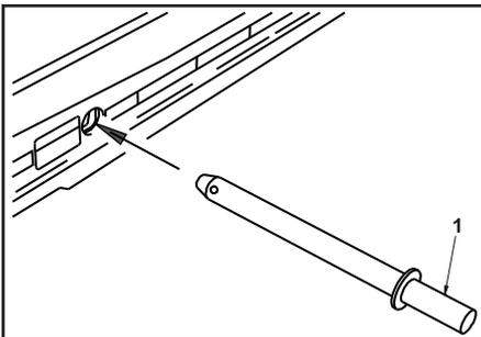
4. Remove the outrigger pins from the storages compartments. Install the pins (1) into the inner sections of the outrigger and secure with the retaining pins (2). (Three section outriggers only).
