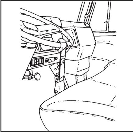
6. After securing the casualty vehicle and before making the final lift, check to be sure that the casualty's parking brake is released, the transmission is in neutral, and the wheels are straight.
