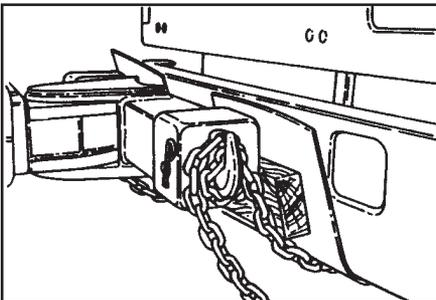
4. Attach hook-up chains to the casualty vehicle. Fasten the chains in the hooks on the end of the adapters and safety wrap the chain around the bottom of the hook as shown. Secure the remaining chain. The use of rubber mats and wood blocks may be required to protect the casualty vehicle.
