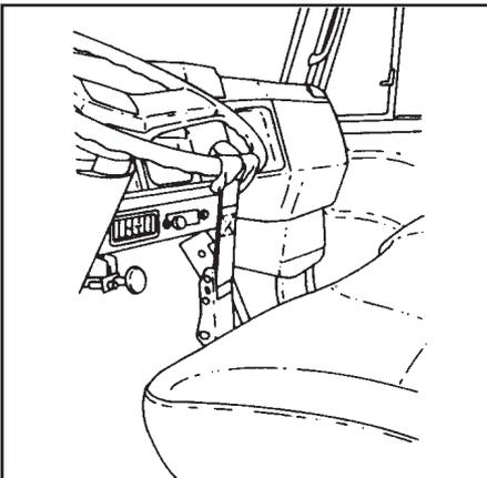
6. It is recommended that the steering wheel of the casualty vehicle be secured by a steering wheel strap for any front or rear tow.
