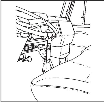
6. After securing the casualty vehicle and before making the final lift, check to be sure that the casualty vehicle's parking brake is released, the transmission is in neutral, and the wheels are straight.
