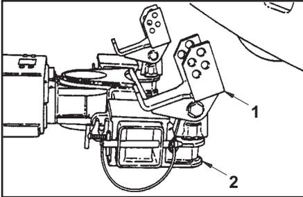
1. Insert the spring lift brackets (1) into the receivers (2) that you previously installed on the crossbar.
