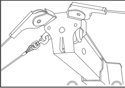
10. DO NOT EXCEED THE WORKING LIMIT OF THE WIRE ROPE. Wire rope ratings can be found on the placard on your unit or in Section 7.1 of this manual. If a heavy lift or pull is to be made exceeding the wire rope working limits, additional cable lines will be necessary.
