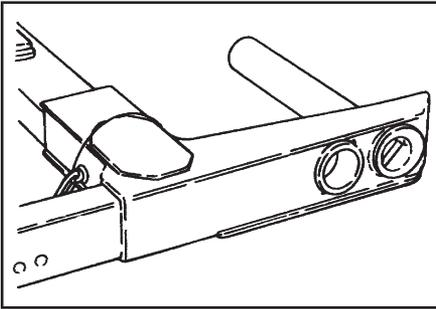
5. Retract the tube inward to the loading position so that the end of the tube will clear the tires.
