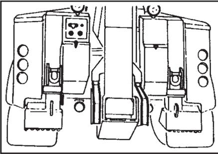
2. Confirm that the recovery vehicle is positioned properly and rests on firm ground. Properly set the midbody outriggers. The rear outrigger/spades can be lowered to provide additional support as required.
