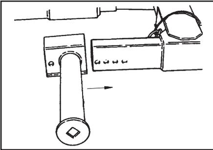
6. Slide the arm weldment over the end of the grid and adjust to the desired position for loading.
