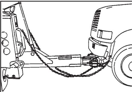
10. Be sure to maintain sufficient ground clearances with the bottom of the casualty vehicle.
