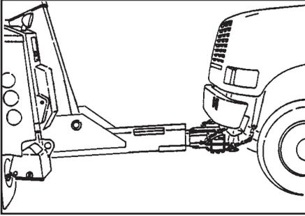
7. With the casualty vehicle in neutral and the parking brake released, the underlift can be raised, lowered, extended or retracted. All of these movements are hydraulically controlled.
