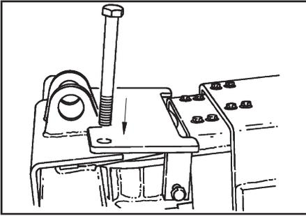
3. Install the retaining bolts thru the keeper bracket and into the adapter. Using a wrench, tighten the retaining bolts until snug.
