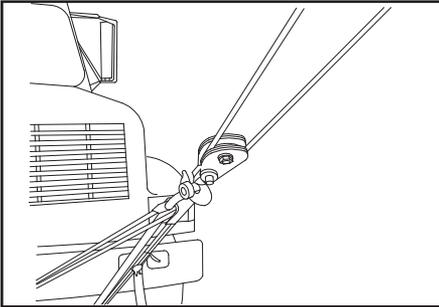
12. The use of snatch blocks and multiple lines will allow you to pull and stabilize the recovery vehicle.
