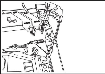
15. Using the winch controls, unwind enough wire rope to remove the hooks or chains and remove them carefully.
