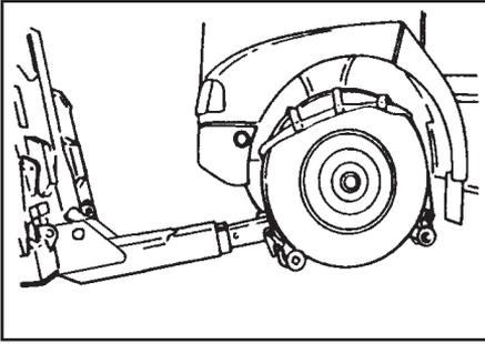
15. Retract the underlift until the casualty vehicle is as close as possible, for the best weight loading, about three (3) to four (4) feet from the back of the recovery vehicle. Leave enough room to maneuver around corners without corner binding or causing contact between the recovery and casualty vehicles.
