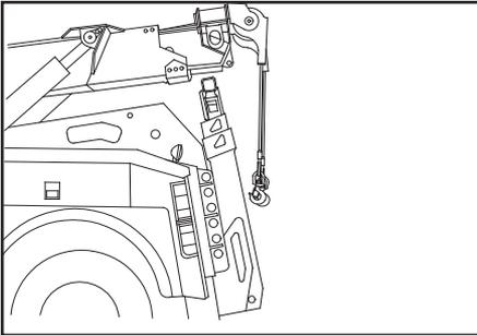
7. Position the boom head by using the boom up, down, in, out and slew left and right levers as necessary.
