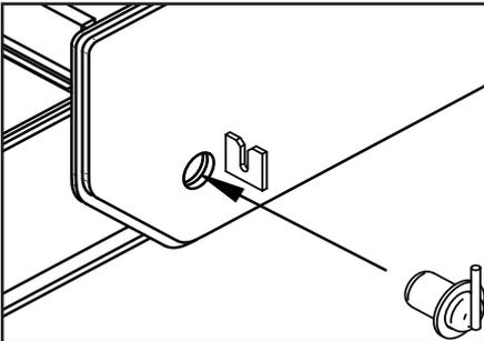
3. Lower the outriggers slightly to gain access to the pinning locations at the upper, inboard ends of the outriggers.
