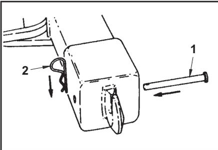
2. Install the retaining pin (1) from the back side of the crossbar through the adapter and crossbar and install the hairpin (2).
