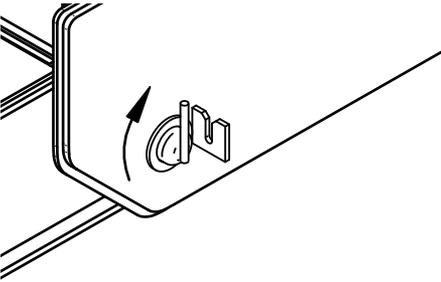
4. Install the pins into the outer sections of the outriggers
