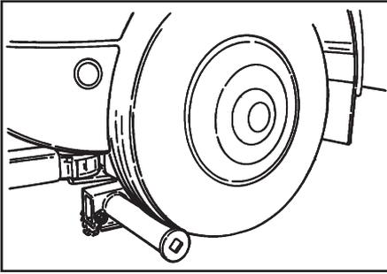
8. Extend the underlift under the casualty vehicle so that the arm makes contact with the front of the tires.
