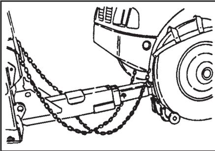
17. Be sure to maintain sufficient ground clearances with the bottom of the casualty vehicle.
