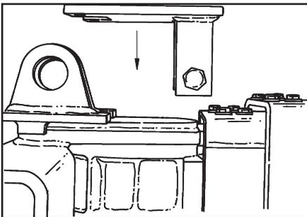
2. Install the keeper bracket down onto the crossbar pivot adapter.
