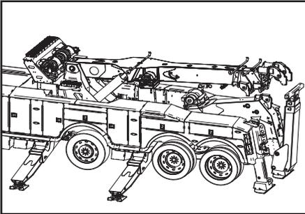
6. Lower the outriggers to the ground. Raise the chassis. Ensure the tires are off the ground a
