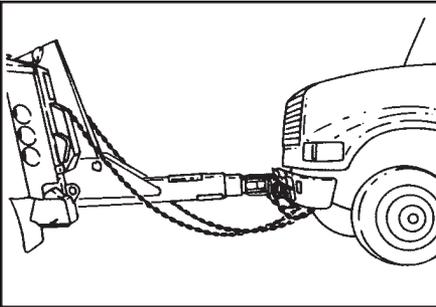
11. Be sure to maintain sufficient ground clearances with the bottom of the casualty vehicle.
