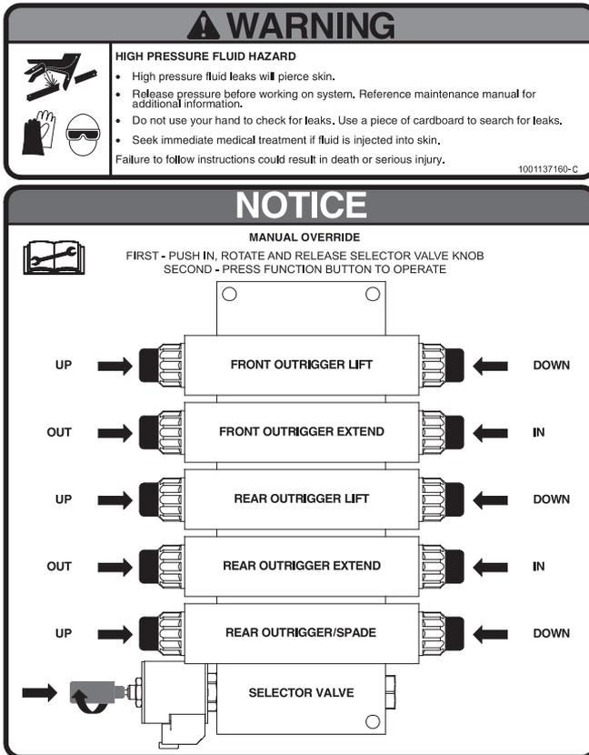
2. Push In, Rotate and Release the "RED" Selector Valve Knob.
