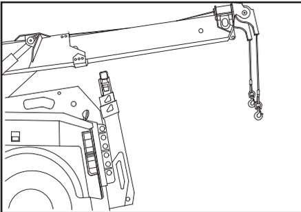
8. Manually, “free-spool” enough wire rope to make the hook-up being sure that a minimum of five (5) wraps remains on the cable drums.
