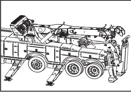
9. Lower the outriggers to the ground. Raise the chassis. Ensure the tires are off the ground a
