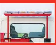
Fully Adjustable Light Pylon Comes standard and easily adjusts to all popular chassis cab heights.
